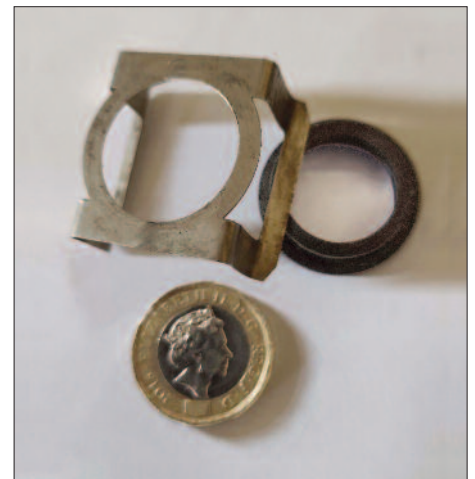
The scale of the Retaining Clip and Seal
